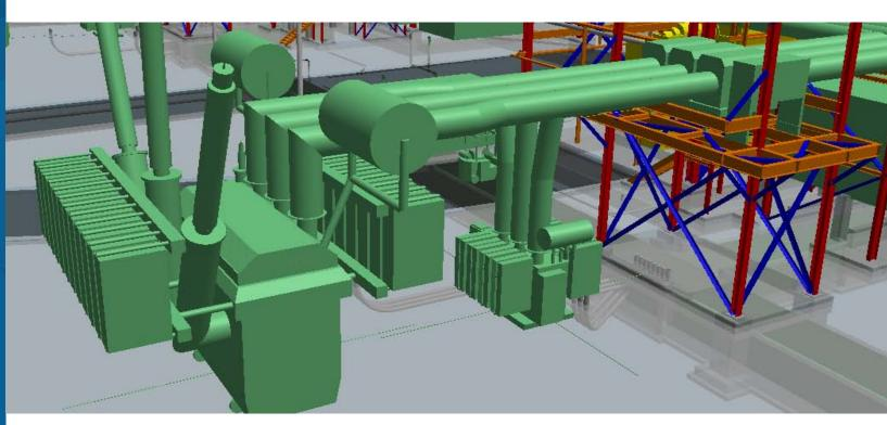
The power will be generated at 11 kV, stepped up to 66 kV through two main oil transformers and evacuated through a new GIS substation within the property of the plant to the National Grid.
